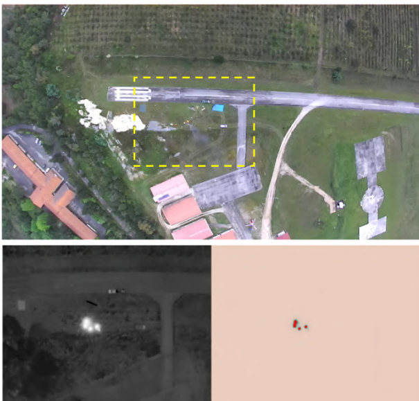
Figure 3. Thermal and visual range samples of data collected in drone flights during fire experiments in an airfield in Lousã, Portugal.
