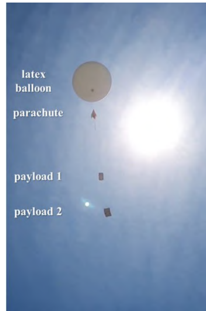
Fig. 3. High-altitude balloon launch and respective payload.
