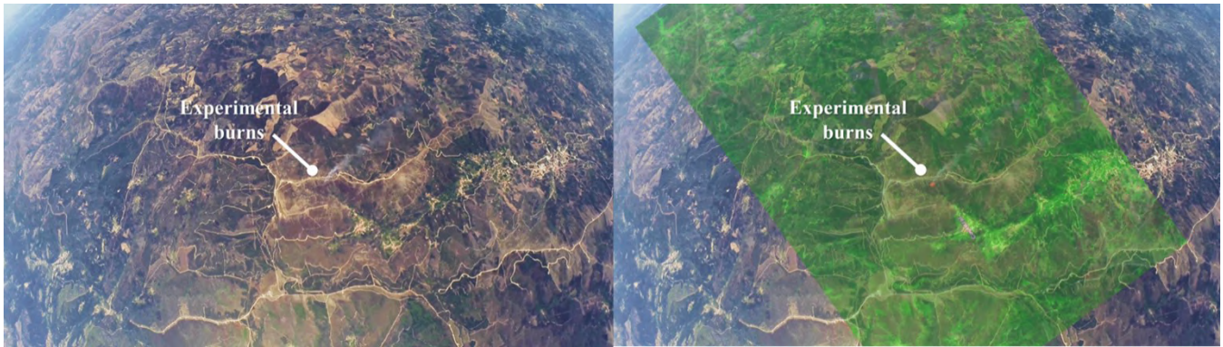
Fig. 5. Balloon aerial view over experimental burns at Coentral, on the 15th May, at 8500 m altitude (left) and Copernicus Sentinel-2 MultiSpectral Instrument data for the corresponding time, where the hot spot is clearly identified in the satellite data in red (right).
