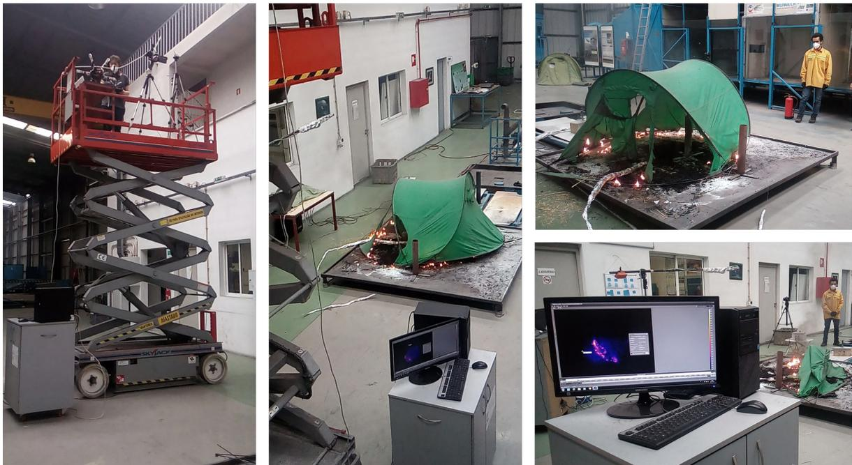
Figure 10.4: Experimental setup for the burning of a tent.
