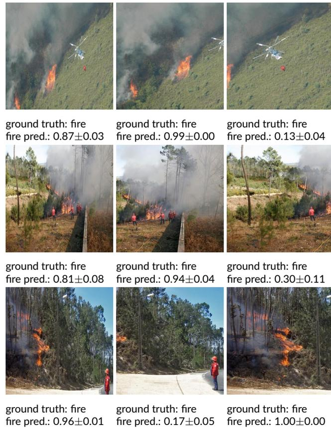
Figure 9.16: Examples of false negative classification associated with fire pattern spatial location on the image borders.
