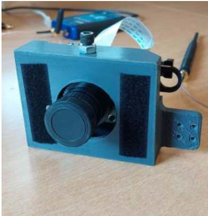
Figure 4.36: Front view and back view of the complete package (Raspberry Pi, Camera, and Modules).
