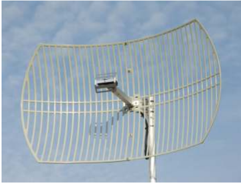
Figure 4.28: 2.4 GHz grid dish Antenna and its radiation pattern on the horizontal plane.
