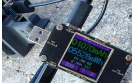
Figure 4.44: USB voltmeter/ammeter with a result of 1070maAh after one hour.
